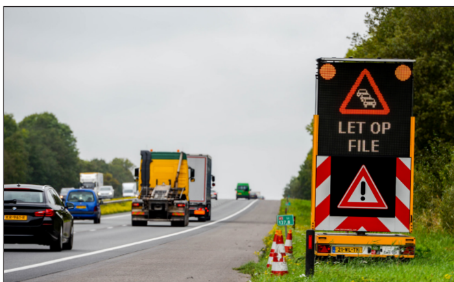
Traffic detection activated on a VMS-trailer
